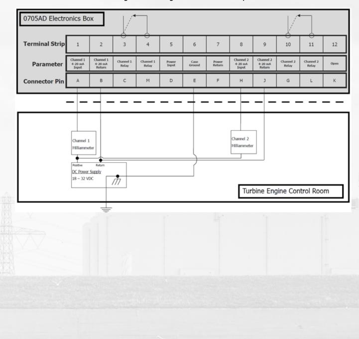
Figure 12 Configuration for 4-20 Loop
