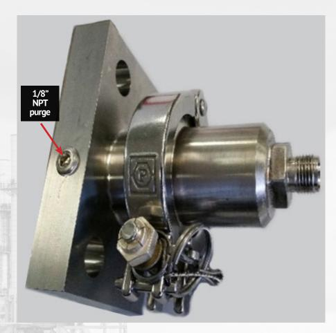
**Note:** In climates with high relative humidity or in applications where engines are operated in peaking service, a bleed air purge line of 1/8" NPT is included within the standard assembly and can utilized if required. The standard assembly comes with a 1/8" allen pipe plug fitted. This feature allows compressor discharge pressure (CDP) air to be used to remove moisture from the FSA optical surfaces.
