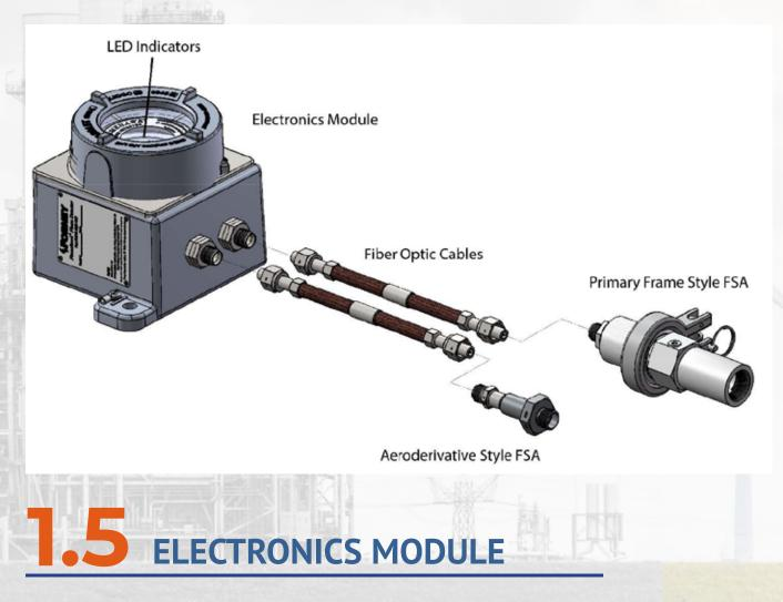
The electronic circuitry is mounted in a modified NEMA 3, 4, 4X, 7(B,C,D), 9(E,F,G) explosion and weatherproof cast aluminum enclosure consisting of a housing and a cover. The cover contains a window for viewing the LED arrays and is sealed with a heavy glass window and gasket. The cover is threaded into the housing and securely sealed with a Nitrile O-ring.
