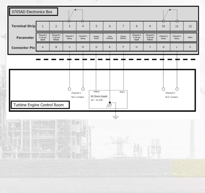
Figure 13 Configuration for Relay Output
