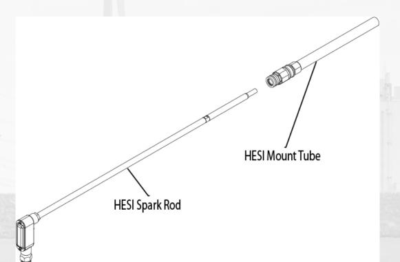
Figure 3 HESI Mount Tube with Quick Disconnect Packing Gland
