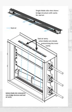
The air seal system is designed to maintain temperatures below OSHA requirements for confined spaces. Two (2) 200% capacity fans (one primary, one backup) help maintain the seal air to the damper when in the closed position. Plus to reduce seal air requirements, Forney's damper uses a flexible seal pack to provide sealing between the blade tips.
