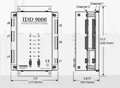
The PM IDD 9000 is available as single or dual channel. The dual channel has a separate, identical PCB motherboard for each channel. Each board contains six connectors on the side panels. Dual channel shown, bottom board is removed on single channel configuration.
