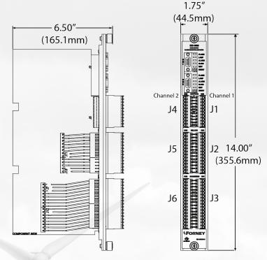
The RM IDD 9000 is a dual channel amplifier with a separate identical CPU Processor for each channel. The right side is for Channel 1 and the left side is Channel 2. The RM IDD 9000 is designed for installation into an amplifier rack (Part # 404325-02) in an equipment cabinet.
