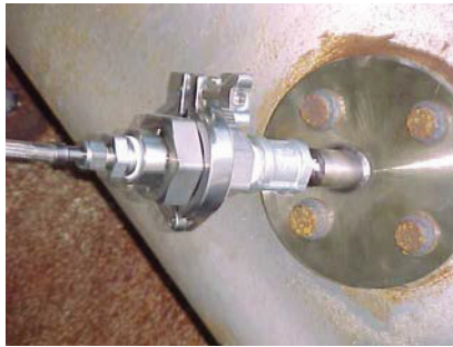
Figure 4 Frame Engine Primary FSA Installation
